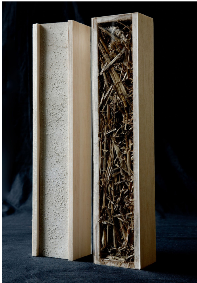
Fig 38: Each straw bale panel consists of a cross-laminated timber frame filled with compressed straw and finished with render for a natural look to the external face, (Make Architects, 2011)
