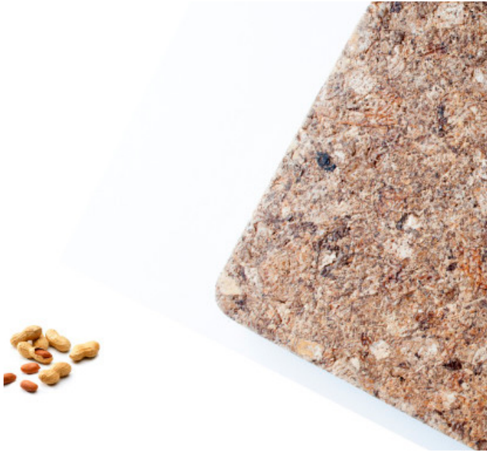
Fig 8: Kokoboard Peanut Shell is a biocomposite board made of waste peanut shells, (Material District, 2014)
