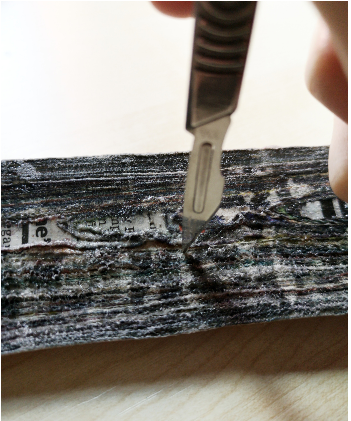
Fig 32: Testing newspaper wood with scalpel (Burton, 2019)
