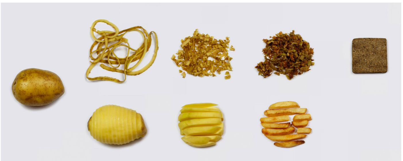
Fig 10: The material is made from a potato peel binding agent mixed with fibres from potatoes, bamboo, wood or hops (Dezeen, 2018)
